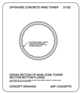
In this concept drawing, a cross section of the base zone tower section bottom flange is shown. The section is slip formed with a fly-ash-based geopolymer cement binder using basalt rebar and fiber reinforcement. (Courtesy: AMF Concepts)
