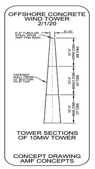
In this concept drawing, sections of a 10-MW offshore concrete wind tower are shown. (Courtesy: AMF Concepts)
