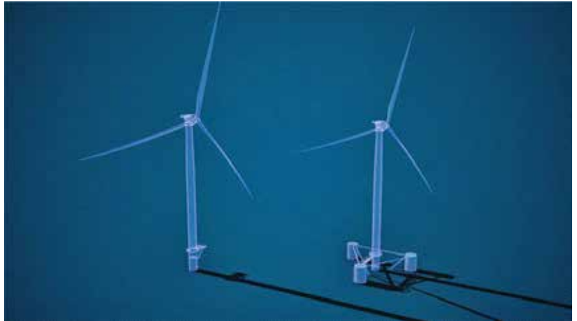
The IEA 15-MW features options for both fixed-bottom turbines and those with floating substructures. (Courtesy: Joshua Bauer, NREL)
