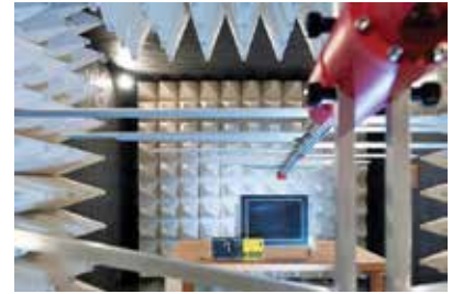
The EMC test facility at Bachmann electronic GmbH: Measurement of electromagnetic emissions. (Courtesy: Bachmann Monitoring)
