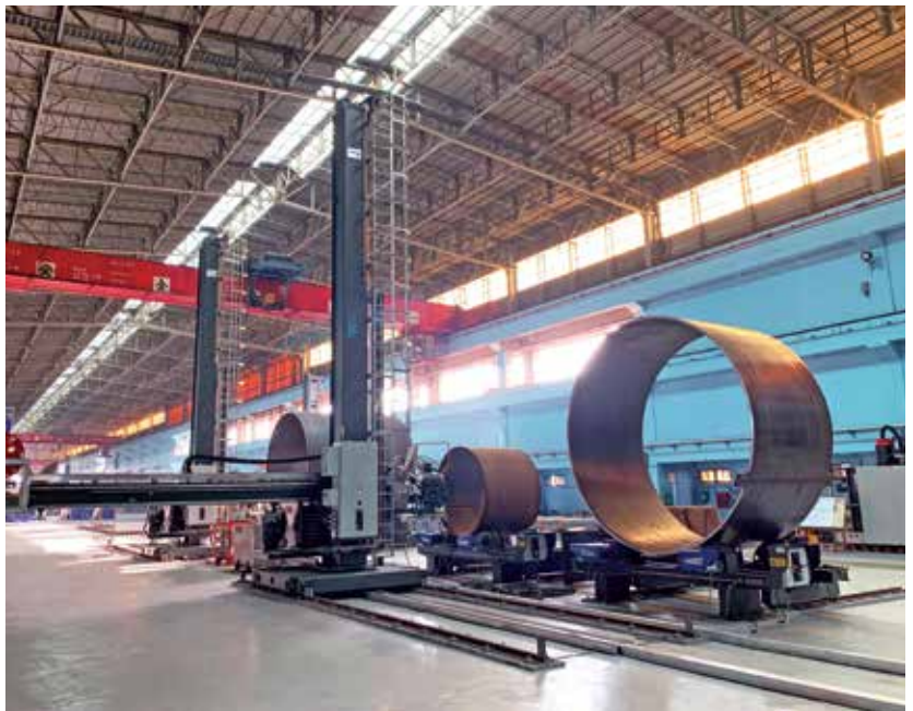
The PEMA production automation lines have the capacity of processing pin piles up to 350 tons and 90 meters. (Courtesy: Pemamek)
