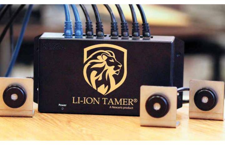
A Li-ion specific system is designed to function as a network of sensors, which enhances its effectiveness in Li-ion off-gas detection. (Courtesy: Nexceris)
