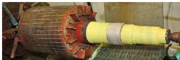
Brush plating equipment is small, lightweight, and portable. (Courtesy: SIFCO ASC)
