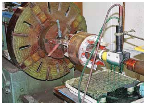
Brush plating presents operators with the answer to two common wear issues seen in wind-turbine generators, bearing seat damage, and slip ring wear. (Courtesy: SIFCO ASC)
