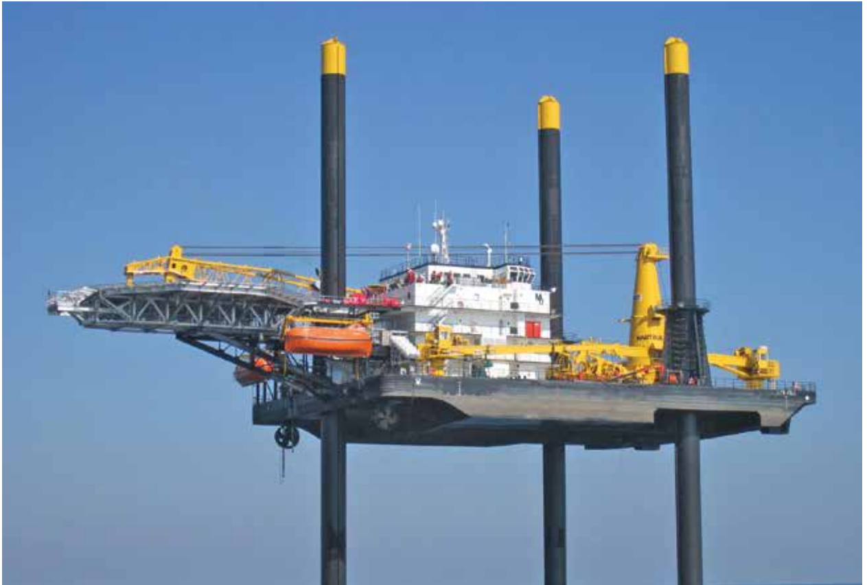
Liftboat Jill is a self-propelled DP2 vessel that can operate in the geotechnical, offshore wind, offshore construction, oil and gas, and cable-repair markets. (Courtesy: Fred. Olsen Windcarrier)
