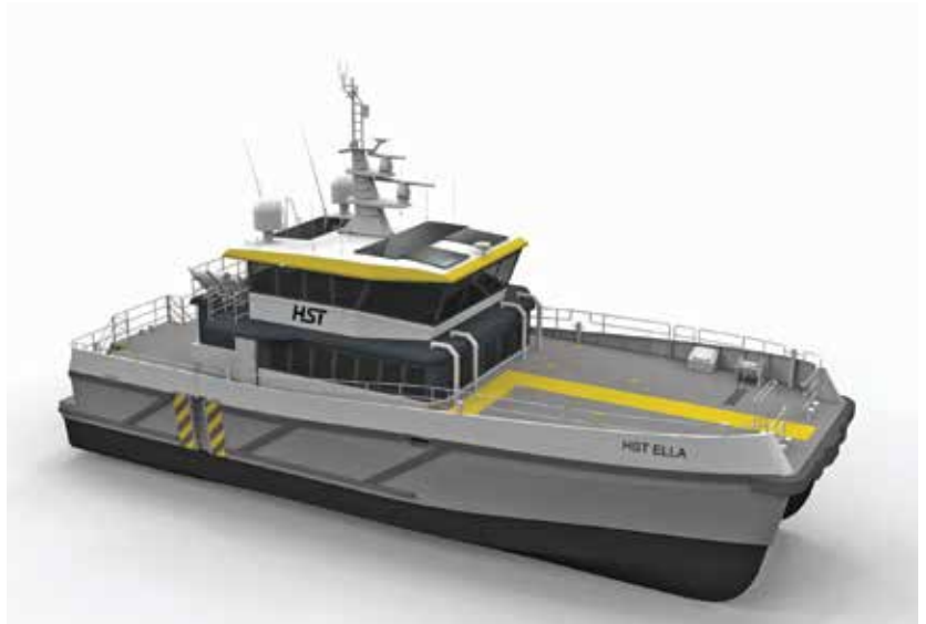
The new hybrid Chartwell 24 design has a unique hybrid propulsion system that incorporates an electric motor alongside a diesel engine, which drive a high-performance changeable pitch propeller (CPP) system. (Courtesy: Chartwell Marine)
