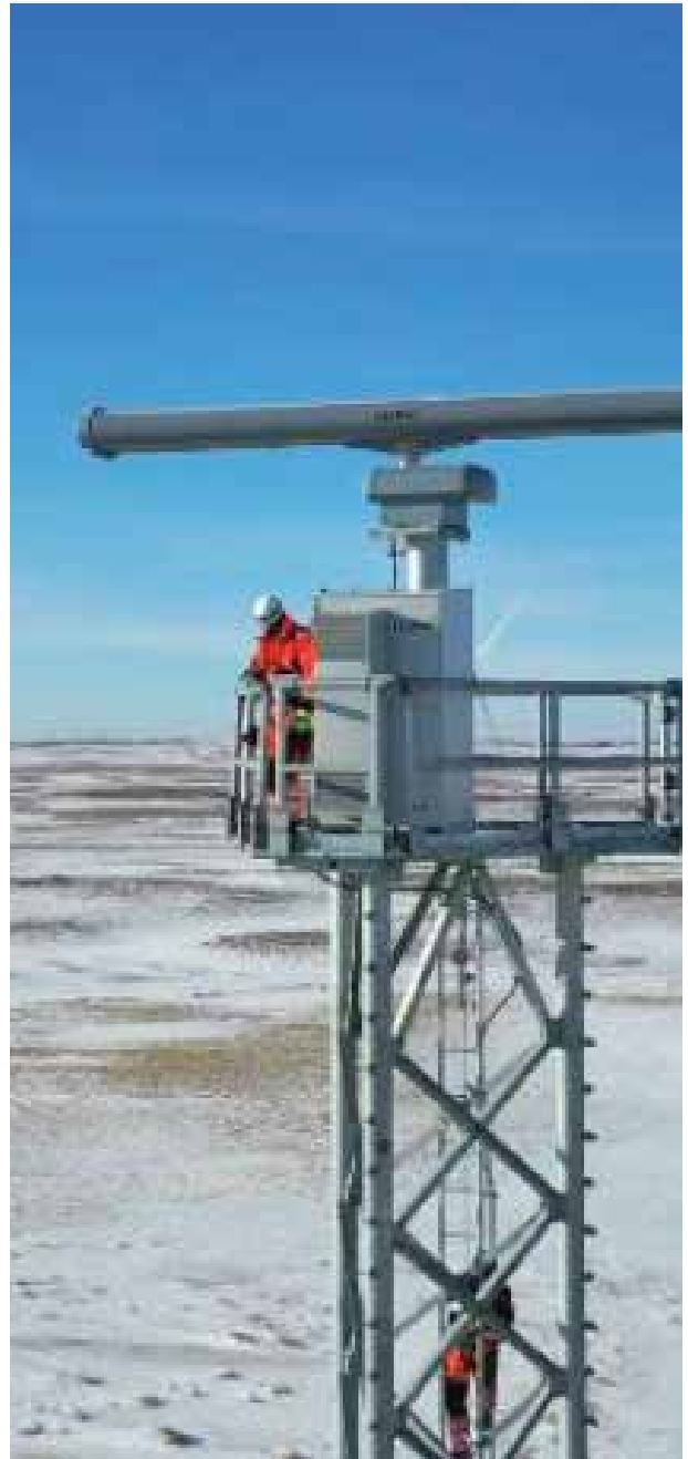
For the ADLS application, Terma uses the SCANTER 5202, a commercial off-the-shelf (COTS), X-band, 2D, fully coherent pulse compression radar. (Courtesy: Terma North America)
