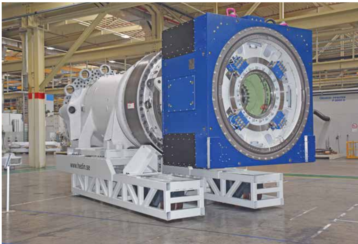
The integrated and modular EnVentus powertrain design includes a main shaft, main bearing housing, a two-stage planetary gearbox, and a permanent magnet generator. (Courtesy: ZF Wind Power)
