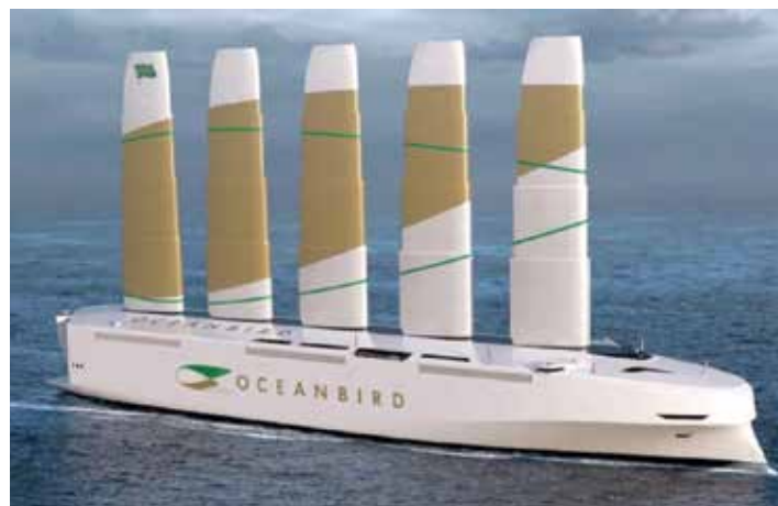
Oceanbird ’s “wings” can be raised and lowered telescopically and will be fully rotational and autonomously controlled. (Courtesy: Wallenius Marine)
