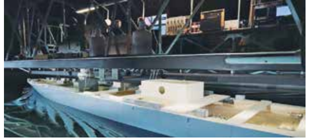
Hydrodynamic testing of a 1:25 scale WPCC hull was conducted at the SSPA towing tank. (Courtesy: Wallenius Marine)
