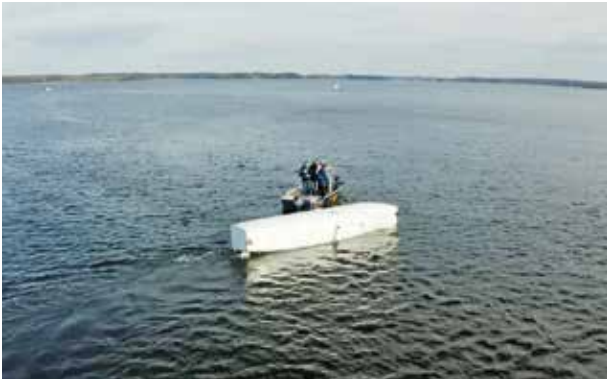
Students at KTH Centre of Naval Architecture built a scale model of the wind-powered car carrier (WPCC) for at-sea testing. The 11 naval design students fabricated a seven-meter WPCC model to validate the ship's center of gravity and also tested the propulsion and steering. (Courtesy: Wallenius Marine)
