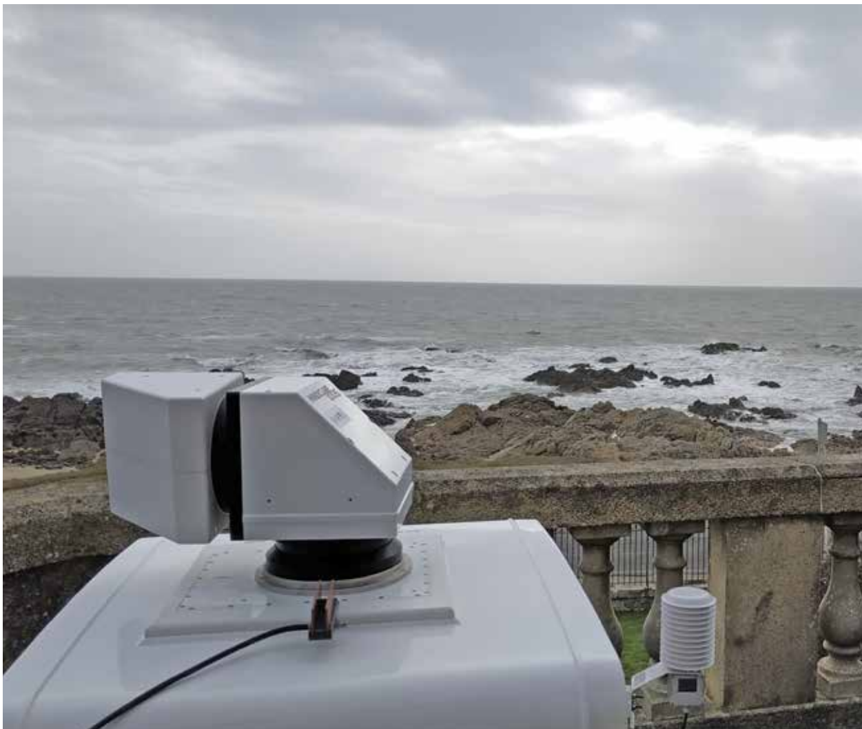
Vertical profiling and scanning Lidars can be mounted on existing offshore platforms or placed onshore at the coastline. (Courtesy: Vaisala)
