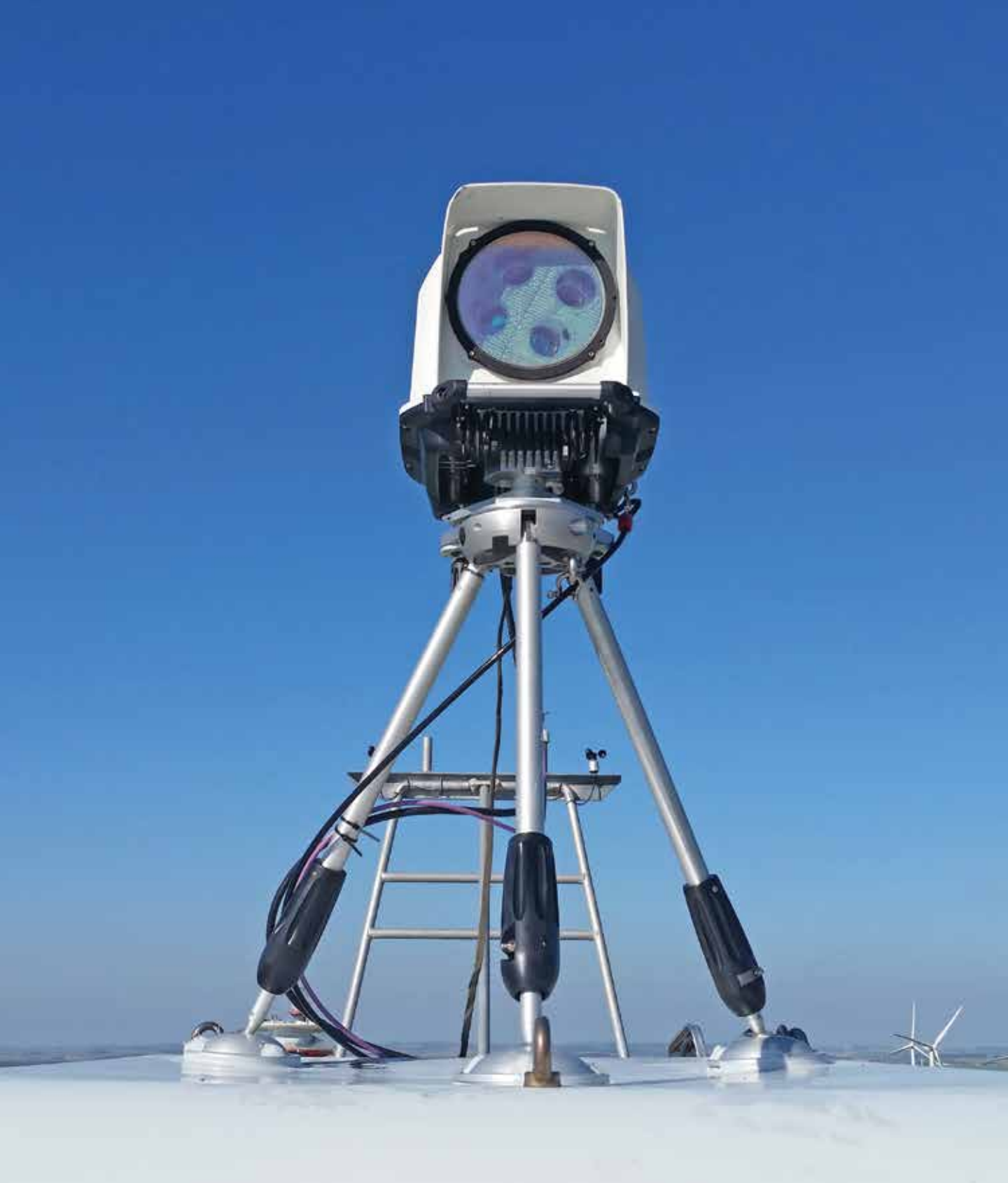
When used for permanent wind monitoring, fixed vertical profiling and nacelle-mounted Lidars can replace met masts and monitor performance and losses when a turbine is stopped or the farm is off the grid. (Courtesy: Vaisala)
