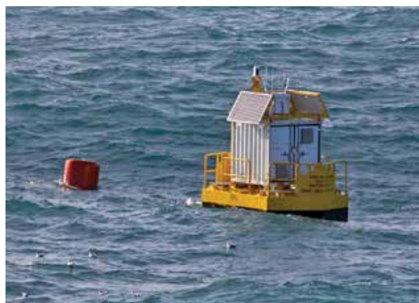
Floating Lidar technology can be deployed for wind-resource assessment nearly anywhere. (Courtesy: Vaisala @ Jacques Vapillon - AKROCEAN GEPS)
