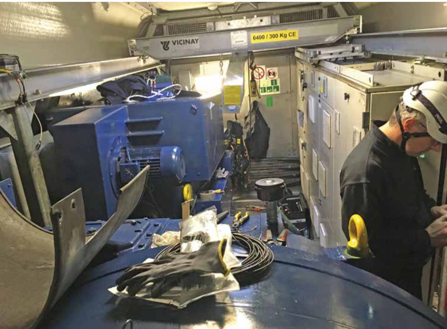
The drive train in the nacelle of a typical wind turbine (2MW). (Courtesy: B&K Vibro)
