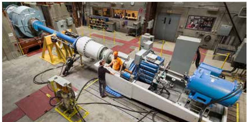
Figure 3: Dynamometer experiment setup of 750-kW wind-turbine drivetrain. Photo by Mark McDade, NREL 32734.
