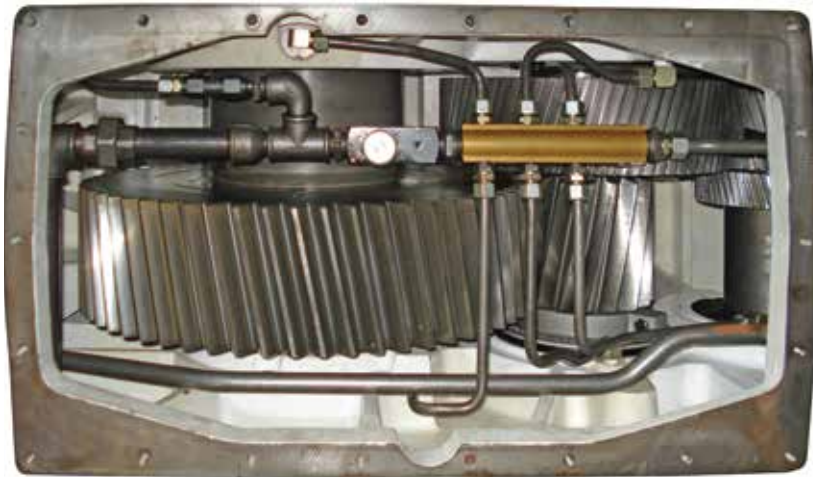
The gearbox of a wind turbine. (Courtesy: SKF)
