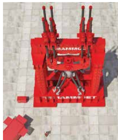
Mammoet’s testing device can test high-capacity equipment to high loads with low risk and minimal impact to operations. (Courtesy: Mammoet)
