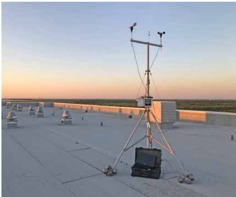
Cup anemometers are widely used to measure wind speed and direction. (Courtesy: Dr. Shu Dai)
