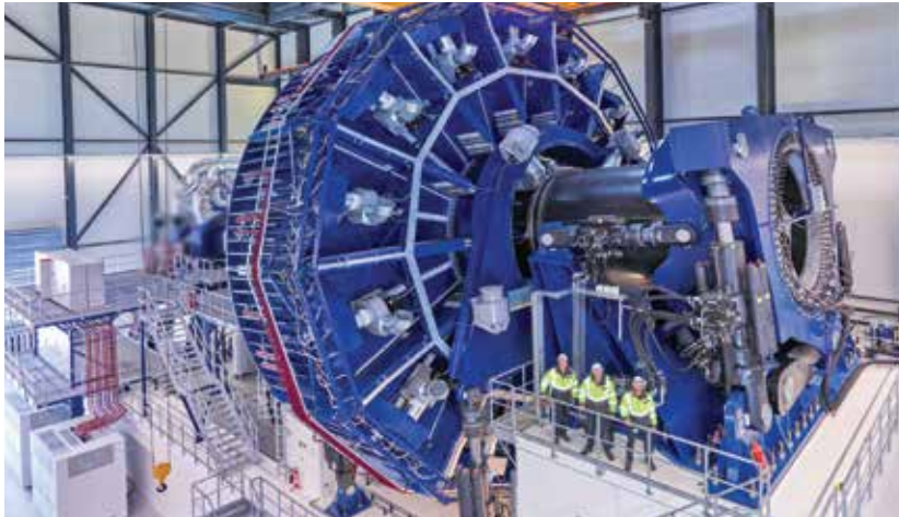
The HALT XL test bench is mounted on a 30-meter-long concrete base and features a 25 MW drive motor that is 15 meters in diameter. (Courtesy: R&D Test Systems)
