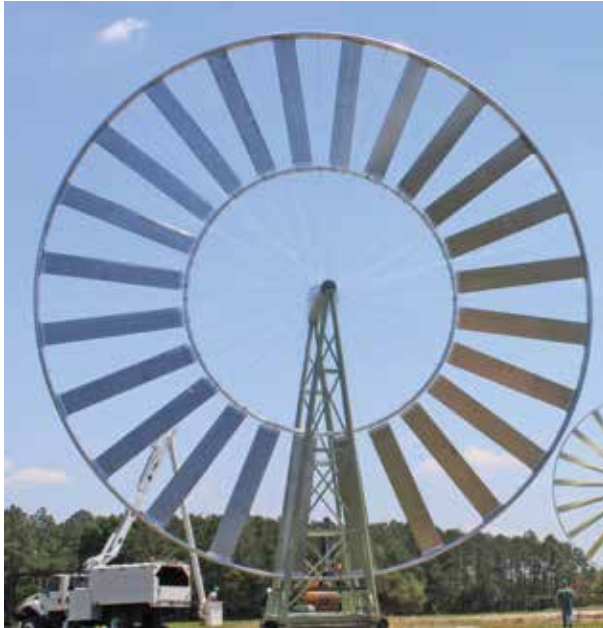
Currently, the Williams Turbine design has been tested with 15- to 25-kW models, with a 1-MW test model being built with a 30-meter diameter. (Courtesy: CryomatiKs)
