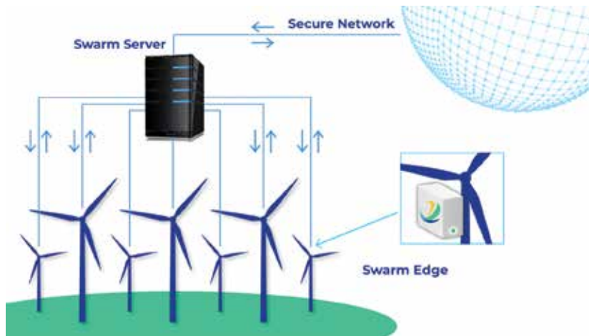
Swarming combines hardware and software as an integrated system to help owners unlock value by allowing turbines to communicate with and learn from each other. (Courtesy: WindESCO)
