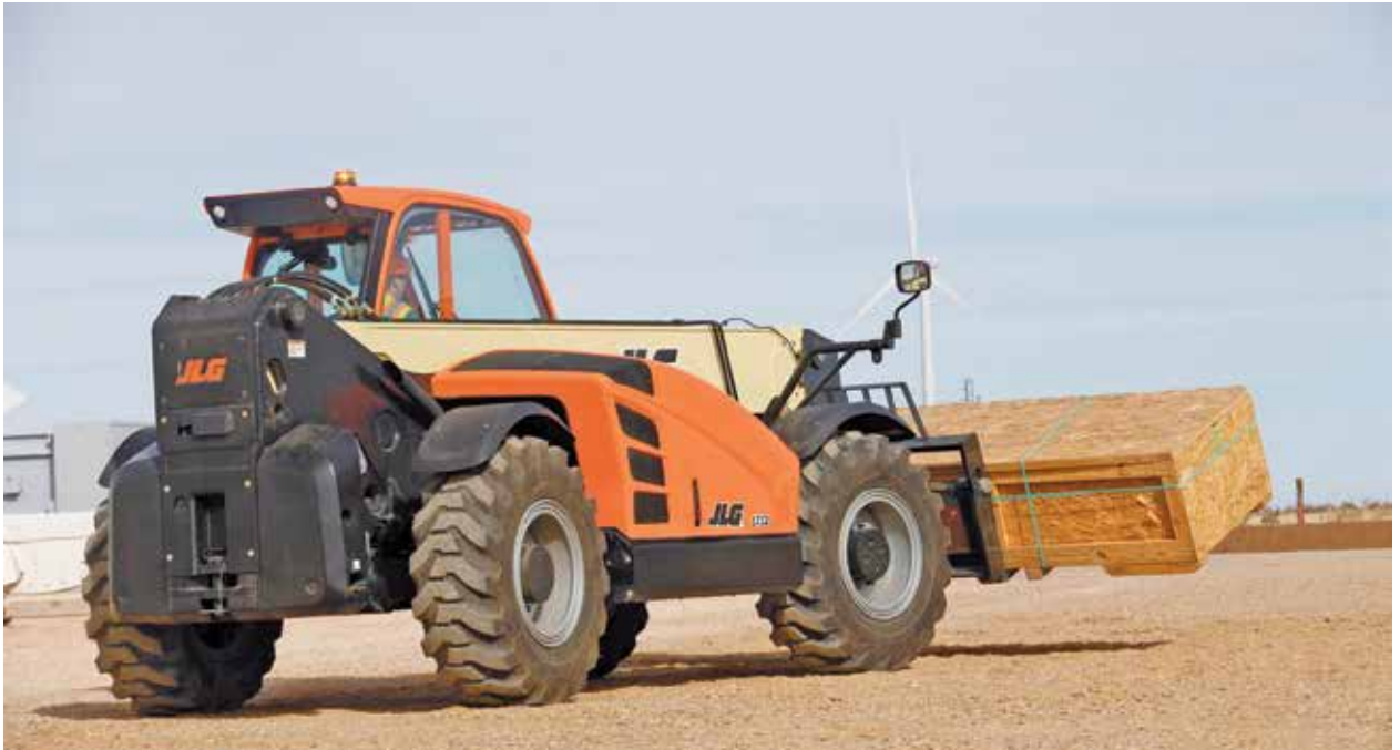
In wind-farm construction, if the operator wants to move one of the blades, or a piece of the tower, a high-capacity telehandler would be used. (Courtesy: JLG Industries)
