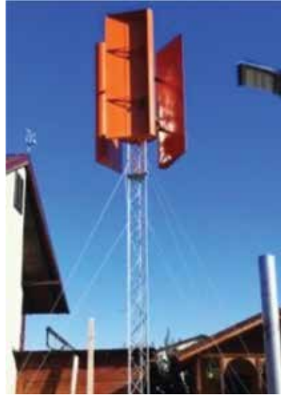
Figure 14: Lenz wind-turbine installed.
