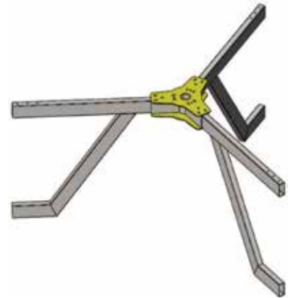
Figure 3: The arm system used for supporting the blades.
