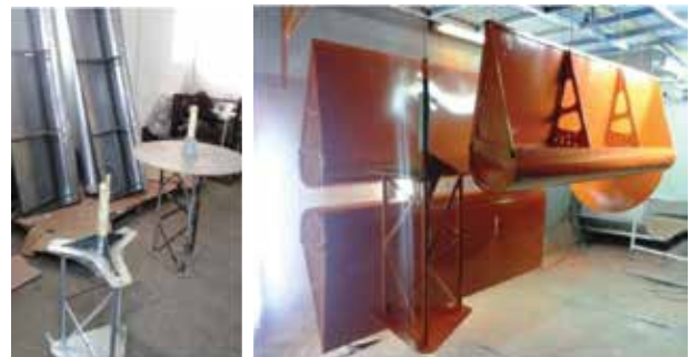
Figure 9: Blades and upper parts from the main pillar before and after the painting procedure.
