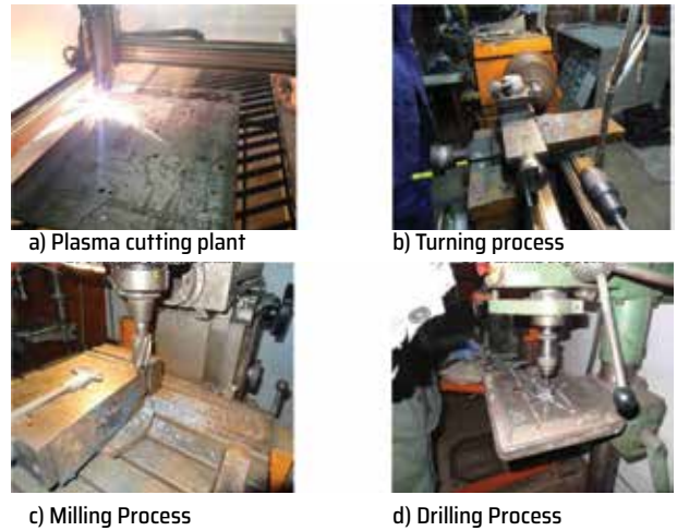
Figure 6: Metal machining processes employed in the manufacturing of the semi-fabricates for the Lenz wind turbine.
