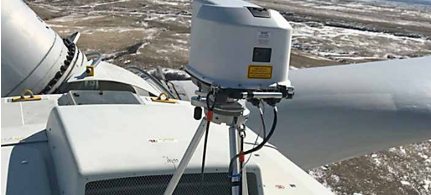
WindCube Nacelle is a laser-based, remote-sensing device that can be easily installed on top of a wind turbine. (Courtesy: Leosphere)
