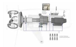
Operating with a modern condition monitoring and predictive maintenance strategy that uses state-of-the-art sensors and algorithms helps to minimize unplanned outages and maximize energy output and revenue generation. (Courtesy: Emerson)
