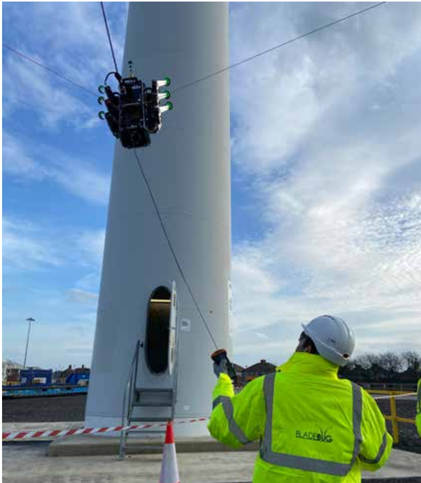
The processes required to rig and operate the BladeBUG can be managed by operations technicians with basic GWD Working at Height training. (Courtesy: BladeBug)
