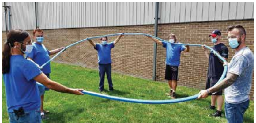
System Seals' first “Super VORTEX” seal with an inside diameter of 3.8 meters. (Courtesy: System Seals)
