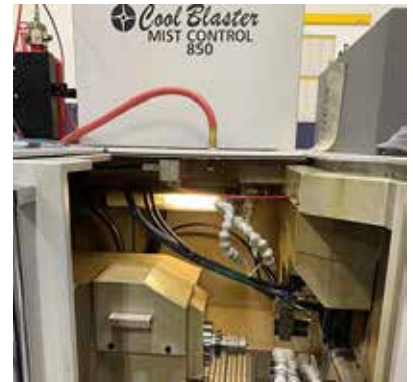
Firetrace systems contain specialized gas or powder, designed for putting out fires, called suppression agents. (Courtesy: Firetrace)
