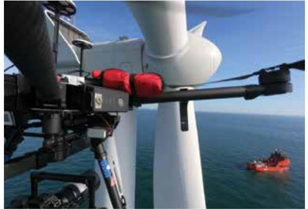
Ventus Group’s AI and machine-learning techniques can detect irregularities in the rotor performance and appearance such as blade damage and bending or twisting differences. (Courtesy: Ventus Group)
