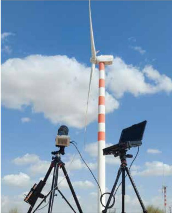
Ventus Group has developed proprietary image acquisition software and methodology and high-speed, high-resolution camera technology that allows for on-site image processing without the need for interrupting the operation of the turbine. (Courtesy: Ventus Group)
