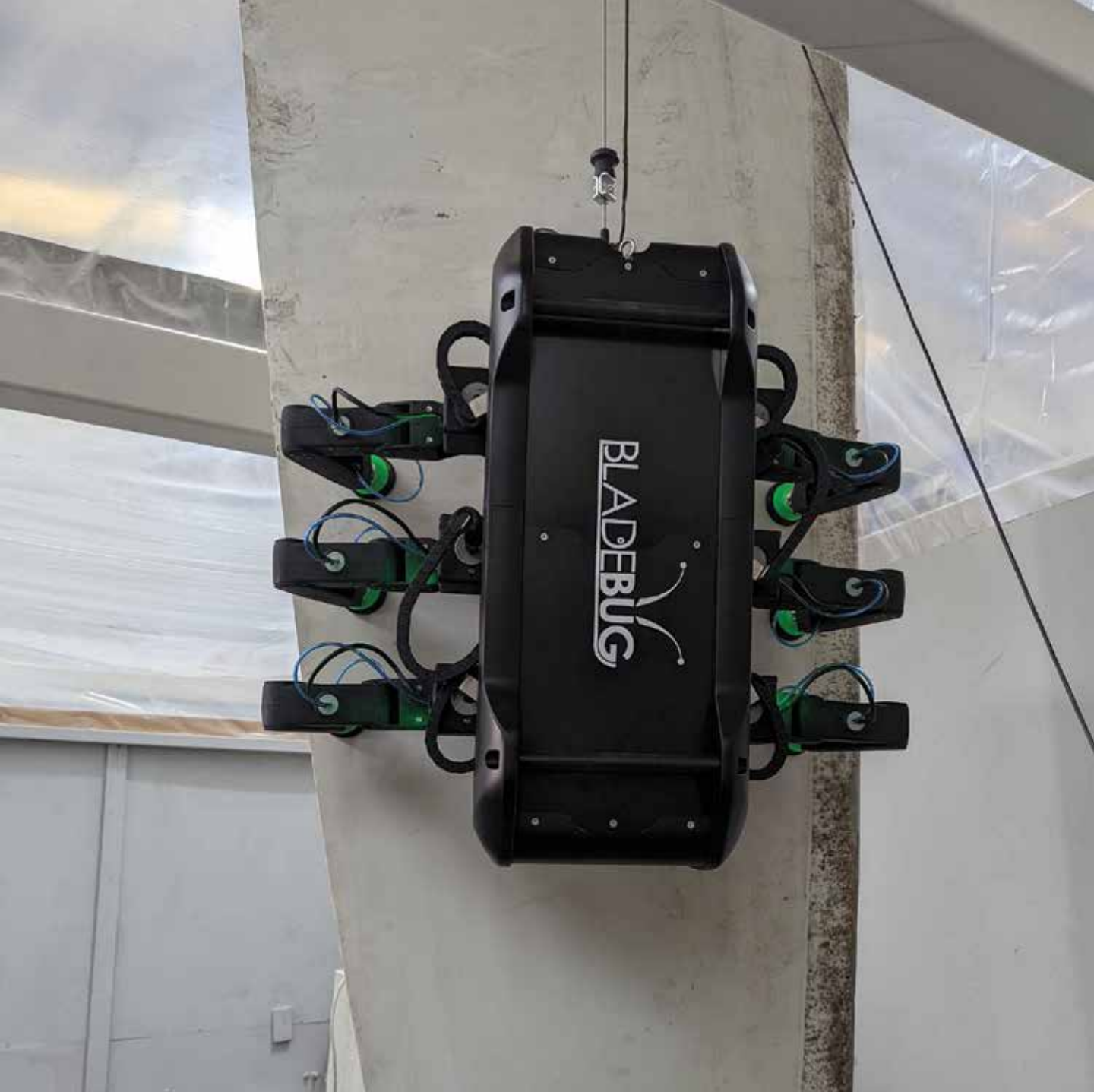
The BladeBUG robot can take away human risk in some common tasks now performed by human technicians. (Courtesy: BladeBUG)
