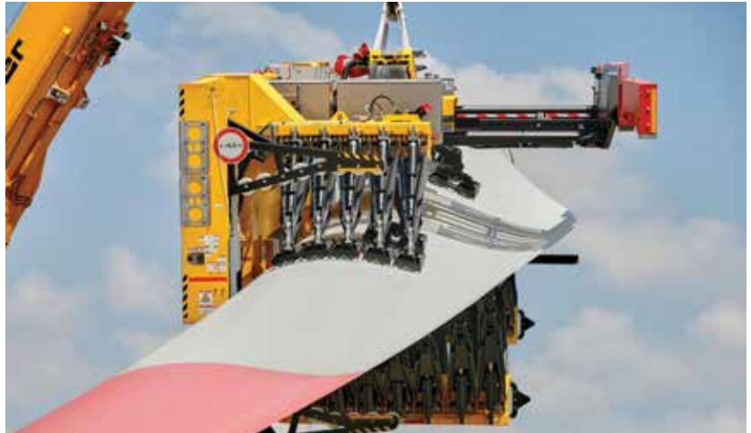
The automatic adaptive blade support of the RBC series yokes is a patent-pending technology. (Courtesy: Ingo Jensen/ematec)
