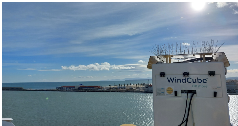
Vaisala WindCube Lidar is integrated into the buoy data acquisition system. (Courtesy: Ocergie)
