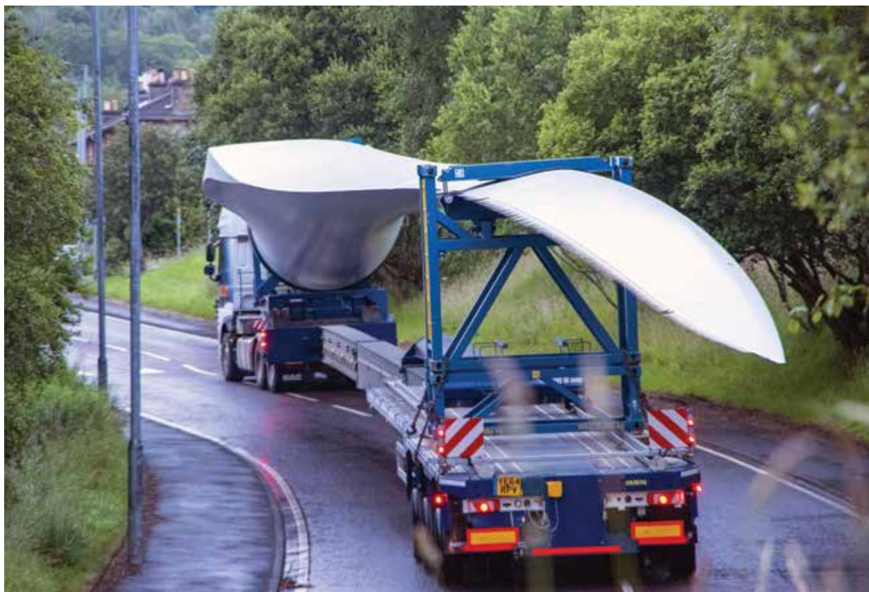
Over the course of the project, Collett handled and transported 150 tower sections, 50 nacelles, 50 hubs, 50 drive trains and 150 blades to South Kyle Wind Farm. (Courtesy: Collett and Sons)
