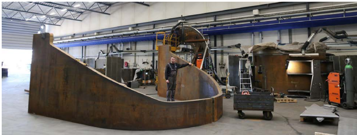
The first steel structure for the new end-of-line test bench has been made. (Courtesy: R&D Test Systems)
