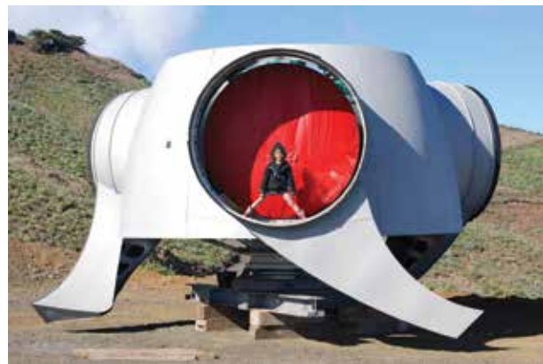
Figure 1: A 5-year-old child stands in a wind-turbine rotor hub. (Courtesy: Erik Streb, CC BY-SA 3.0)
