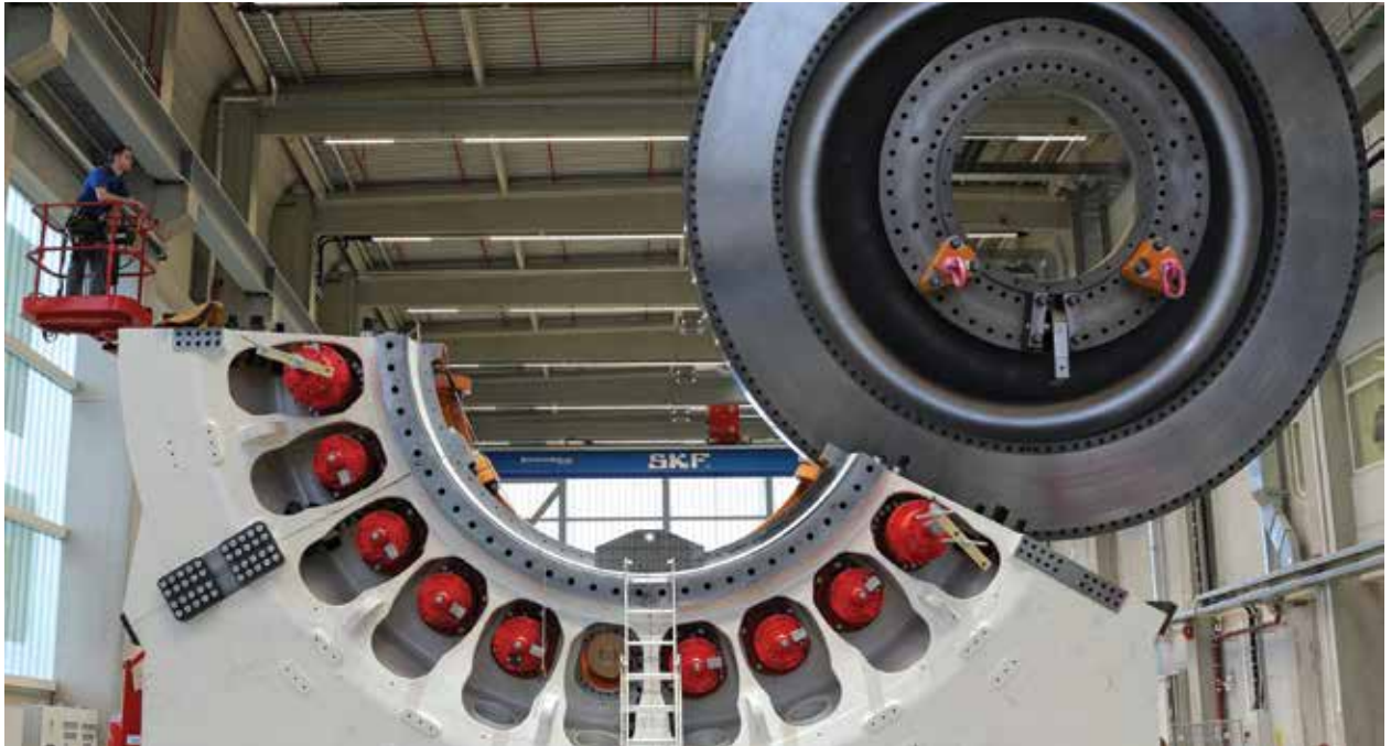
Figure 7: The 125-metric-ton, seven-meter disc is lifted into position in the lower half of a test rig at the SKF Sven Wingquist Test Center in Schweinfurt, Germany. This rig can test bearings up to six meters in diameter, as well as complete bearing assemblies. (Courtesy: SKF)
