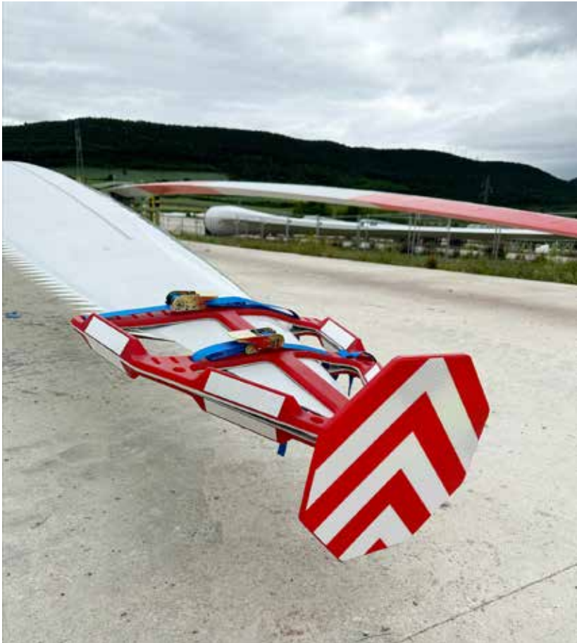
PRO-PAD TIP 1 will meet safety requirements for people near the blade, as well as transporting the blade. (Courtesy: Dansk Gummi Industri)
