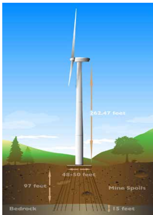
Figure 4: A micropile-supported wind-turbine foundation mitigates the detrimental settlement effects of mine spoils. (Courtesy: Barr Engineering Co.)
