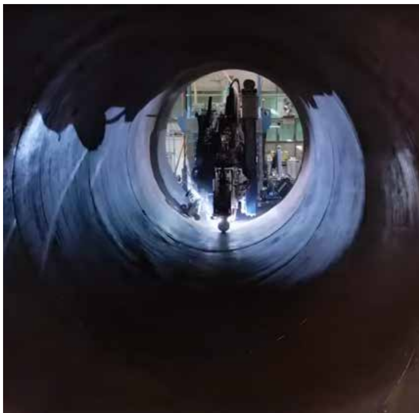
Keystone's tapered spiral welding process brings the speed, quality, and consistency of automated manufacturing to wind-tower manufacturing. (Courtesy: Keystone Tower Systems)
