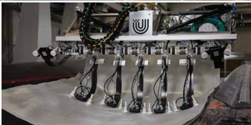
Discrete tape laying over the complete blade system. (Courtesy: Siemens)
