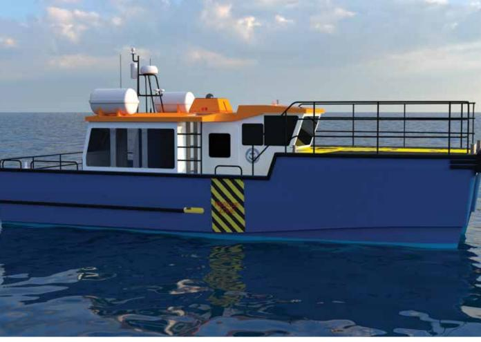
Chartwell's design responds to the increasing demand in the U.S. offshore wind market for low-emissions, cost-effective support vessels, with the catamaran's optimized hull form offering efficient fuel use as well as stability and maneuverability in choppy waters. (Courtesy: Chartwell Marine)
