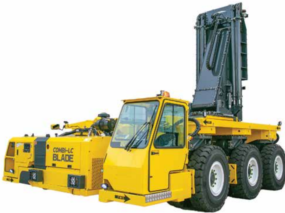
The COMBI-LC Blade load mover is designed to work with any model of blade. (Courtesy: Combilift)
