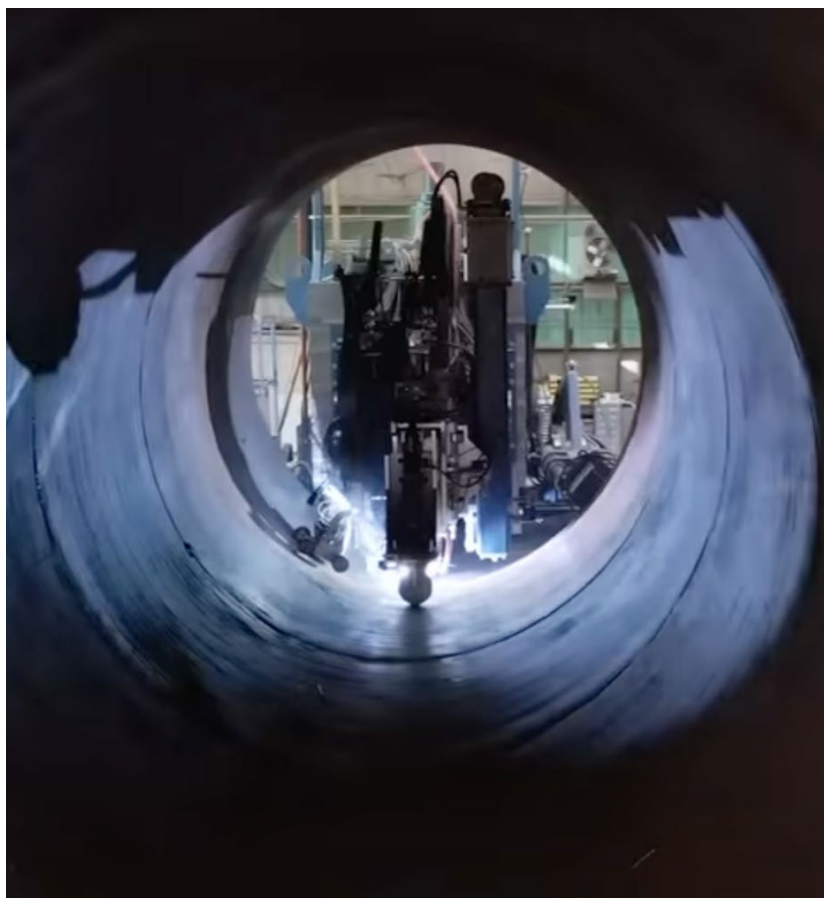
Keystone's tapered spiral welding process brings the speed, quality, and consistency of automated manufacturing to wind-tower manufacturing. (Courtesy: Keystone Tower Systems)
