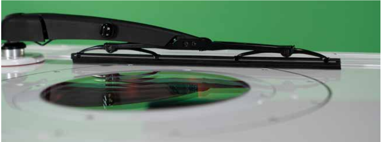
Lidar — light detection and ranging — uses laser pulses to sense wind conditions remotely, providing expanded coverage and flexibility compared to fixed met towers. (Courtesy: Vaisala)
