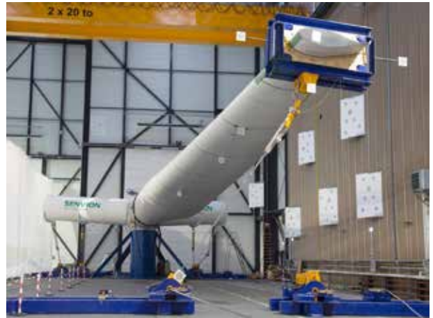
(b) “BEAT2.1,” for 2-meter bearings (at blade root) @Fraunhofer IWES/ Martina Buchholz.
