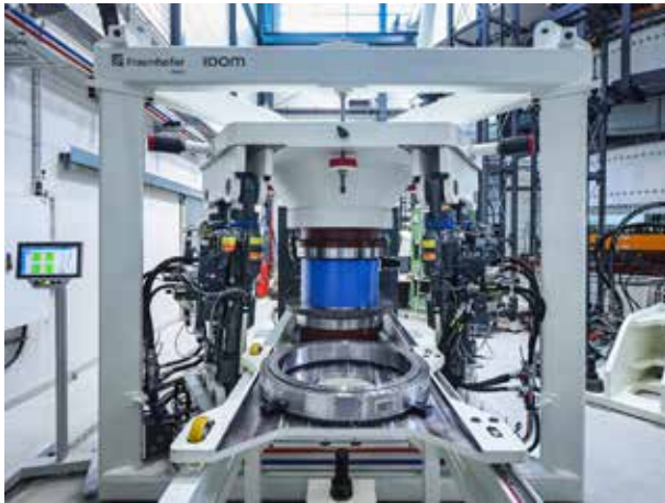
(a) “BEAT11,” for 0.7-meter bearings (in metallic) @Fraunhofer IWES/ Ulrich Perrey.
