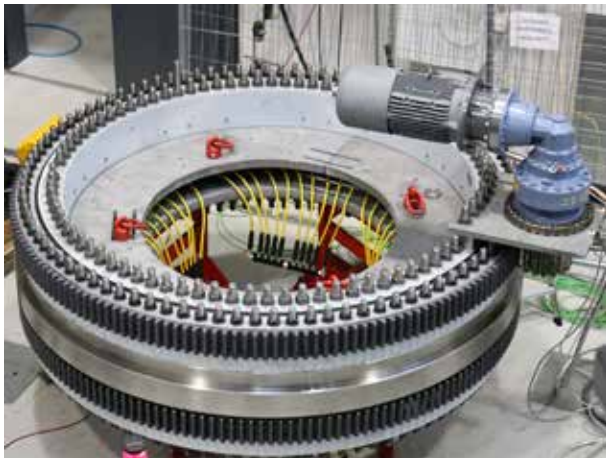
(c) “BEAT2.2,” for 2-meter bearings (in non-metallic gray, with gear teeth on outer ring) @Fraunhofer IWES/Karsten Behnke.
