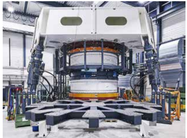
(d) “BEAT6.1,” for 5-meter bearings (in orange) @Fraunhofer IWES/ Marcus Heine.
