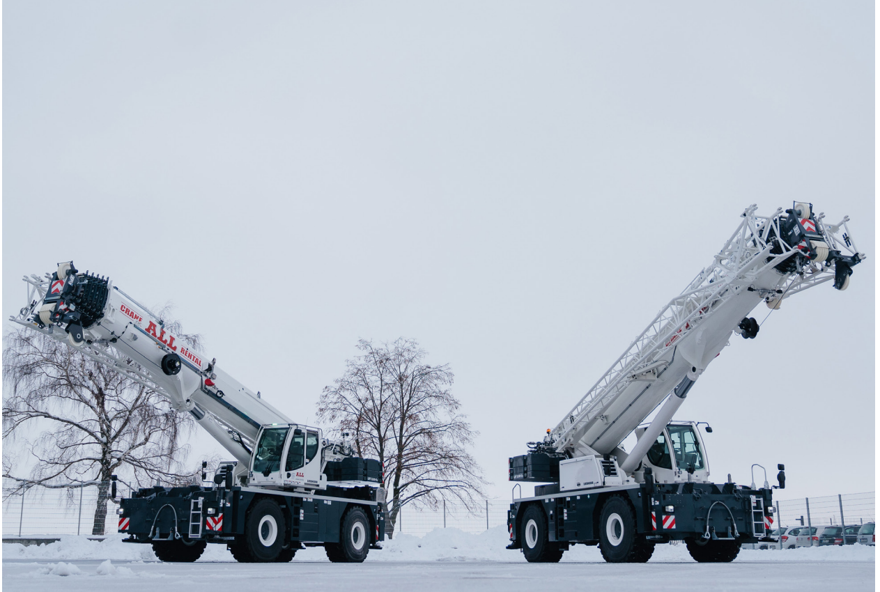
The Liebherr LRT 1130-2.1 boasts the longest telescopic boom of any two-axle RT. (Courtesy: ALL Crane)
