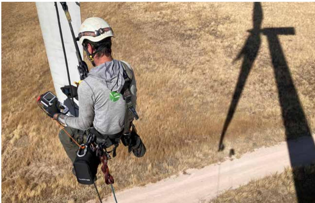
Figure 2: Technician out on a rope using DLRO on a blade. (Courtesy: Megger)
