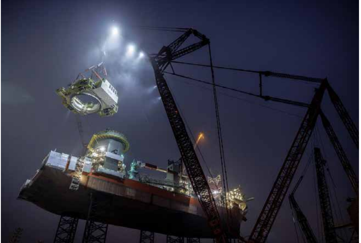
Motus Technology's crane is developed to lift five tons at 30 meters. (Courtesy: Motus Technology)
