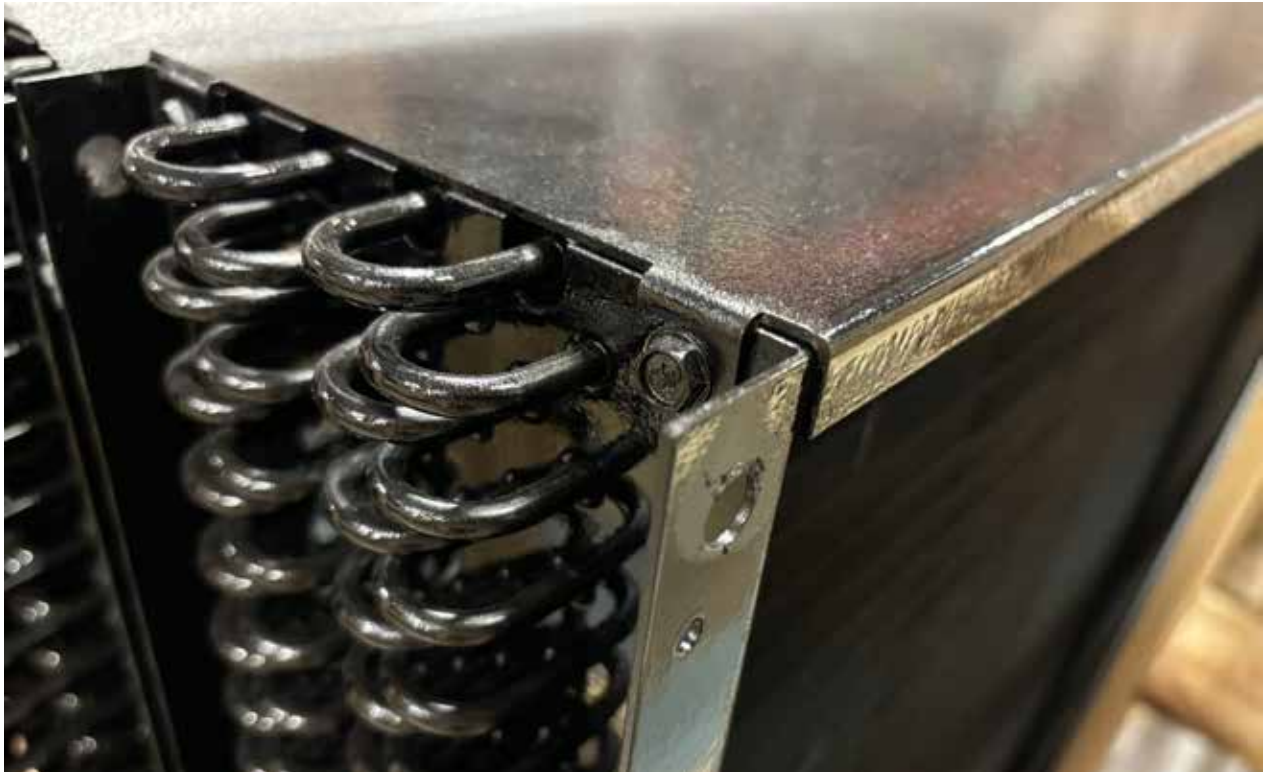
Custom loop thermosyphon hardware. (Courtesy: ACT)
