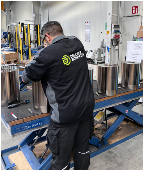
A factory worker completes manufacturing of rotor lock pins for OEM wind turbines. (Courtesy: Dellner Bubenzer Group)
