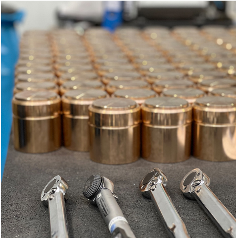
A line-up of barrel pistons and pucks being produced for yaw passive braking system. (Courtesy: Dellner Bubenzer Group)
