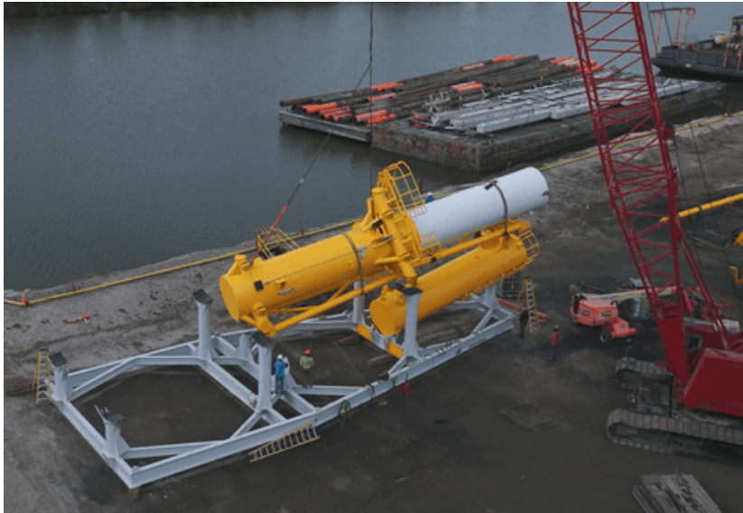
Aikido is working with Norway’s METCentre on a floating wind platform. (Courtesy: Aikido Technologies)
