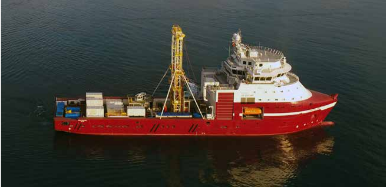
By deploying the Dina Polaris vessel, equipped with geotechnical drilling, sampling, and testing equipment along with an offshore laboratory, Geoquip provided seabed data. (Courtesy: Geoquip Marine)
