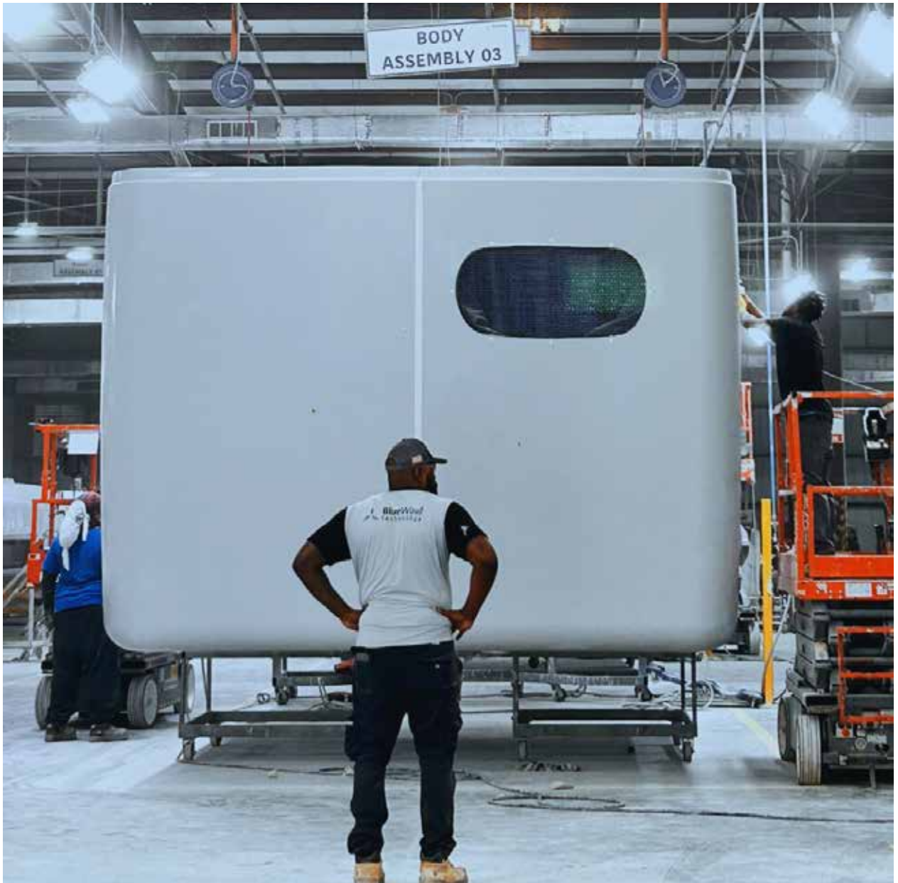
The nacelle covers are made with composite fiberglass and resin and assembled in the BlueWind factory. (Courtesy: BlueWind Technology)
