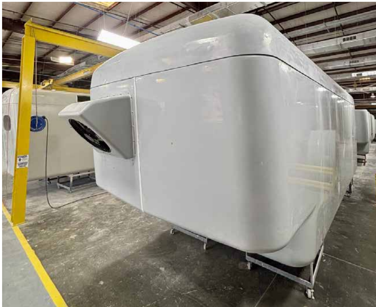
The nacelle covers produced by BlueWind Technology are made with processes called vacuum infusion silicone skin system. (Courtesy: BlueWind Technology)
