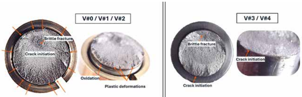
Figure 6: Failure morphology differences between metal & laser coatings.
