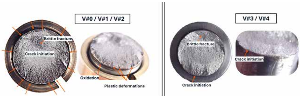
Figure 6: Failure morphology differences between metal & laser coatings.
