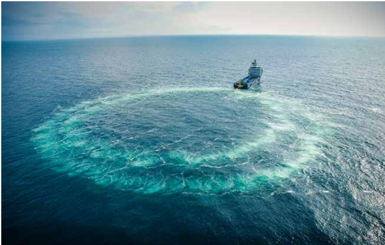
Jaeger Maritime Solutions required a bubble curtain to absorb and disperse sound, safeguarding surrounding marine ecosystems from harmful noise levels. (Courtesy: Jaeger Maritime Solutions)
